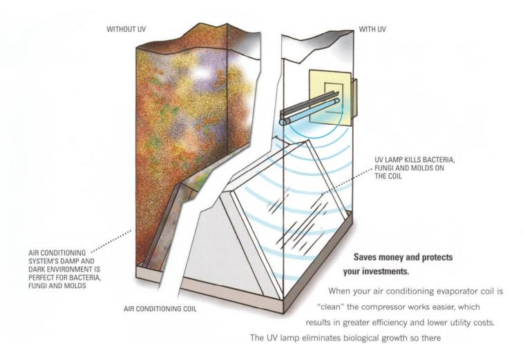
extends the life of your air conditioning equipment. "Keeping coils sanitary - through cleaning and the application of chemicals and/or UV lights - is part of a system-wide approach, which
